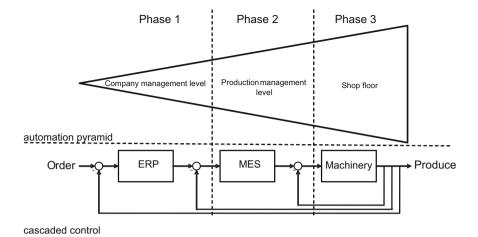
Fig. 4 Automation pyramid in comparison with cascaded control
