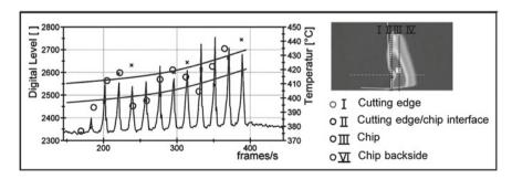
Fig. 5 Reducing calibration variance via location-referenced measurements [7]
