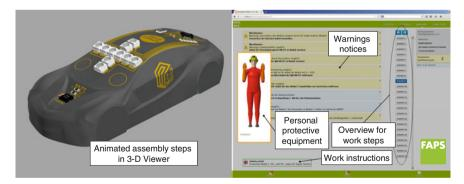
Fig. 19 Showing 3D product assembly models in TeamCenter Visualization Mockup (*left*) and further worker information on a website (*right*)
