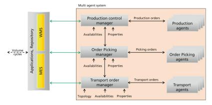
**Fig. 8** Simplified overview of intelligent agents representing the CPS in the SMART FACE project. The data of the volume cycle is centrally stored in a repository. Basic functionalities like a Warehouse Management System and a Manufacturing Execution System are operating as applications on this repository. Software agents for order picking, transportation and production control are interacting with the repository
