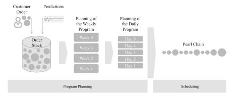
**Fig. 6** Present structure of the program planning process and sequencing in automotive industry (cf. [6]). Customer orders and prediction from sales and market are gathered in the order stock. On this basis, the orders are distributed uniformly on weekly programs first, and on daily programs afterwards. The scheduling stage calculates a specific sequence within the weekly or daily programs, the so-called *pearl chain*
