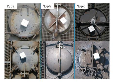
Fig. 1 Dome cover closure types
