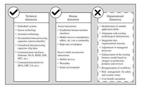
Fig. 1 Dimensions of the successful implementation of industrial cyber-physical systems
