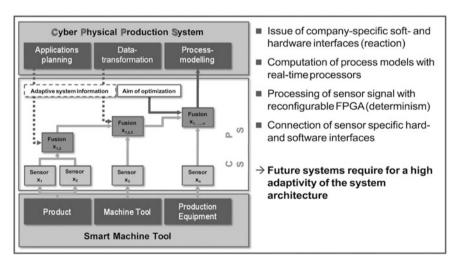
Fig. 7 Cyber-physical sensor system [7]
