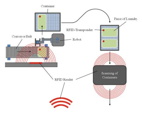
Fig. 6 Overview of the picking setup
