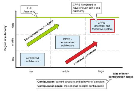
Fig. 8 Autonomy masters the complexity of CPPS
