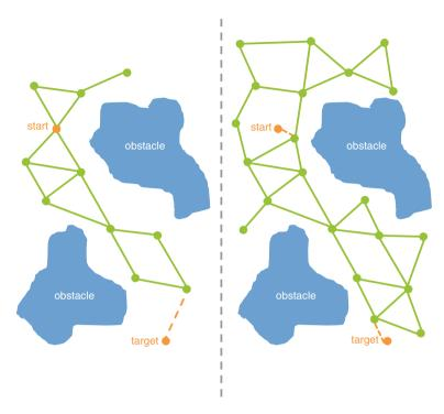
**Fig. 16** Generation of a single-query tree (*left*) and a multi-query map (*right*)
