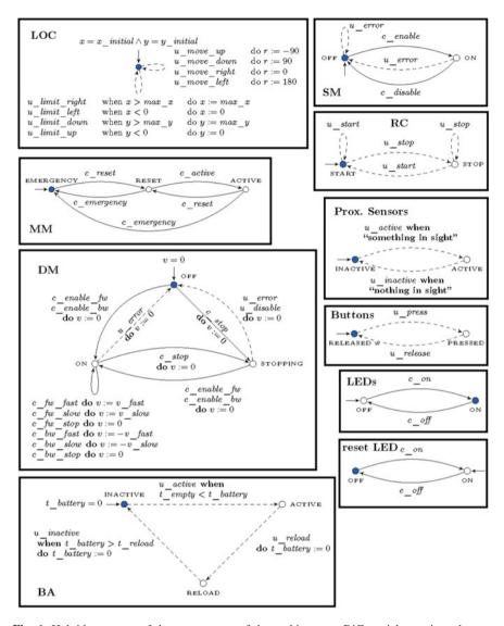
Fig. 6 Hybrid automata of the components of the multi mover. Differential equations that are used to define the values of the continuous-time variables are presented in the appropriate subsections
