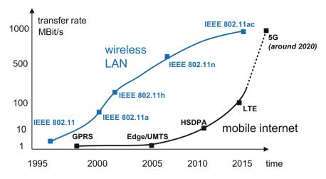
Fig. 2 Transfer rates of wireless LAN and mobile internet technologies (own illustration)
