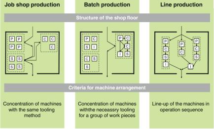
P... paste printing, C... component placement, S... soldering, I... Inspection
