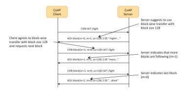
Fig. 9 A CoAP client requests the resource light and receives a block-wise answer. The client requests more blocks until the server informs the client that no more blocks are available
