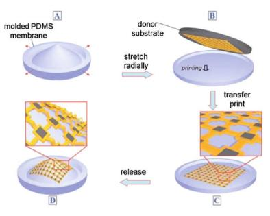
Fig. 5 Deployment of electronic systems onto an arbitrary curvilinear surface via transfer printing. Reprinted with permission from [68]
