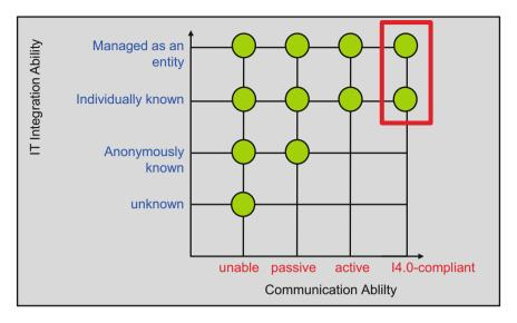
Fig. 6 Classification of an I4.0 component According to [44]
