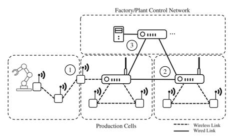
Fig. 3 Communication scenarios between production cells within the factory or across the whole factory site. Individual cells are either (1) connected through wireless links or (2) by multi-homed gateways, connected via a wired link. Ultimately, these are connected to (3) the control and automation network of the factory
