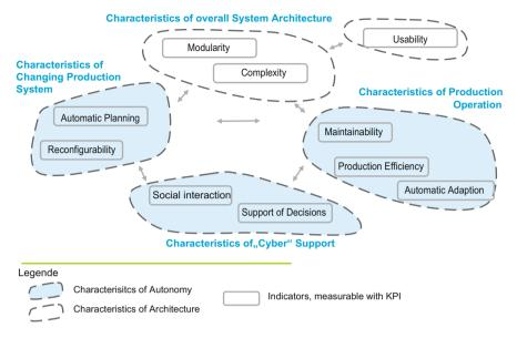
Fig. 9 Classification of measurable indicators towards characteristics of systems
