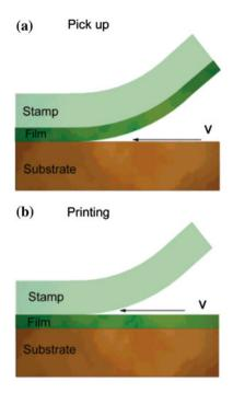
Fig. 2 Diagrams for pickup of a thin film from substrate and printing a thin film onto another substrate. Reprinted with permission from [17]
