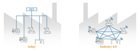
Fig. 9 Change from hierarchical to decentralized systems in an industry 4.0 environment
