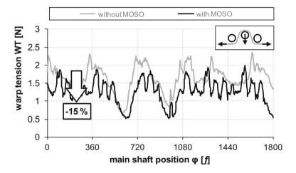
Fig. 4 Comparison of warp tension with and without MOSO
