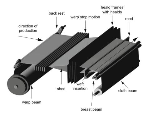
Fig. 1 Setup of a weaving machine [1]
