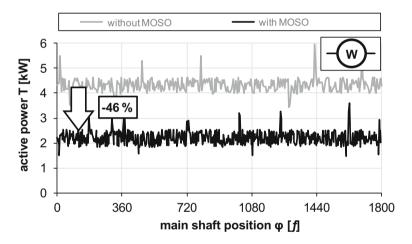
Fig. 6 Comparison of active power consumption with and without MOSO
