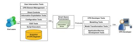
Fig. 7 The architecture for a user-driven cyber-physical system
