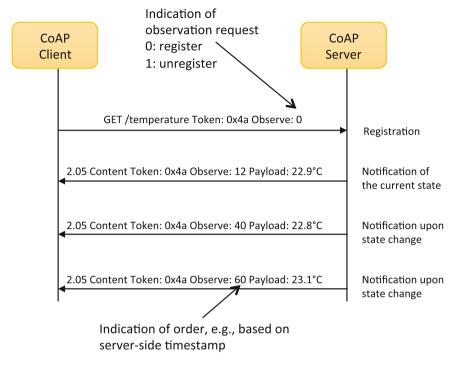
Fig. 10 A CoAP client registers to the resource temperature at a CoAP server. The server replies with several notifications whenever the temperature changes (cf. [26])
