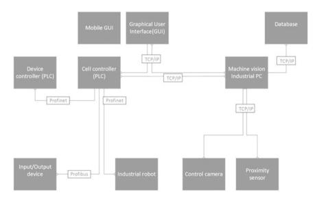
Fig. 3 Communication structure of automation
