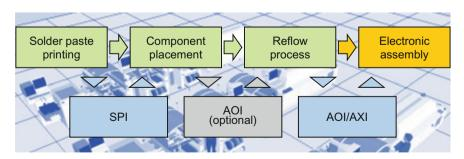
Fig. 1 Process chain in electronics production with optional inspection steps [16]
