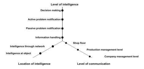
Fig. 2 Classification model for the manufacturing environment (based on Meyer et al. [13])
