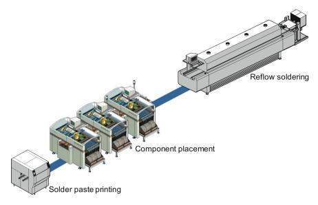
Fig. 6 In-line structure of an SMD assembly line
