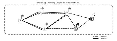
**Fig. 6** A communicates with F using the graph with  $ID\ 1$  (dotted line). To send a packet on that graph, A can either forward to B or C. Ultimately, following this graph will end at F. Similarly, in order to send data to D, A can use the graph 2 (solid line)
