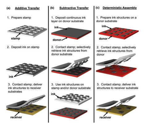
Fig. 1 Schematic of three transfer printing schemes. a Additive transfer delivers 'inked' materials at regions that come into contact with the target substrate. b Subtractive transfer results in patterned material on donor substrate, as well as inked material on stamp for additive transfer, as in (a). c Deterministic assembly involves removal of selected structures from the donor substrate, followed by a printing onto a receiving substrate. Reprinted with permission from [16]
