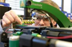
Fig. 7 Smart glasses as CPAS in assembly tasks
