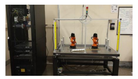
Fig. 8 A fully assembled discrete manufacturing robotics enclave
