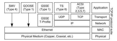
Fig. 7 The communications stack of IEC 61850
