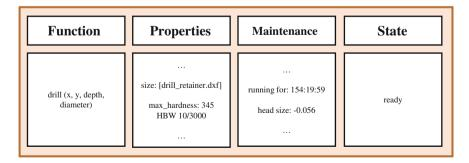
Fig. 2 Example for a possible metal drill's memory contents
