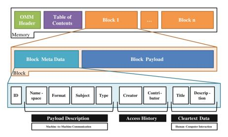
Fig. 4 Data model for object memories based on W3C object memory model incubator group (OMM-XG)
