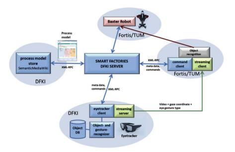
Fig. 4 Intelligent user interface architecture
