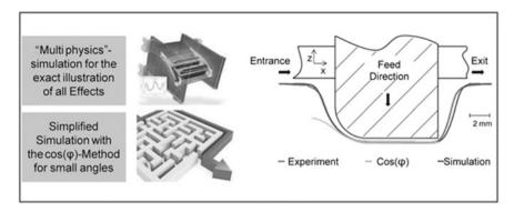
Fig. 8 Modelling concepts for reducing calculation times [5]
