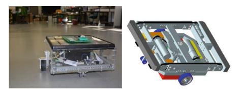
Fig. 13 ASWC with circuit board (left), CAD model of an ASWC (right)
