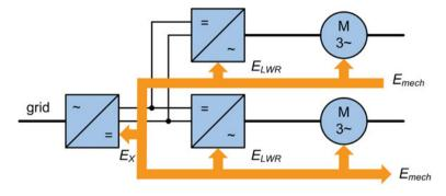
Fig. 4 Two motors connected to a DC circuit
