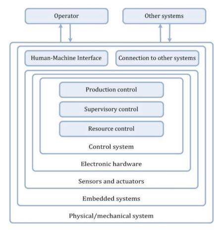
Fig. 1 Positioning of supervisory control
