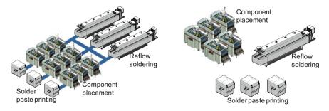
Fig. 7 Online structure (left) and offline structure (right) of assembly lines in electronics production
