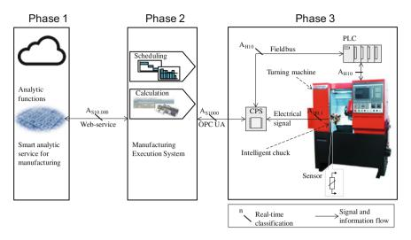
Fig. 5 CPS for a turning machine
