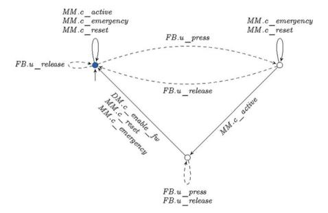
Fig. 10 Requirements for button handling. Shown is the automaton for handling of the forward button. A similar requirement automaton is needed for the handling of the backward button
