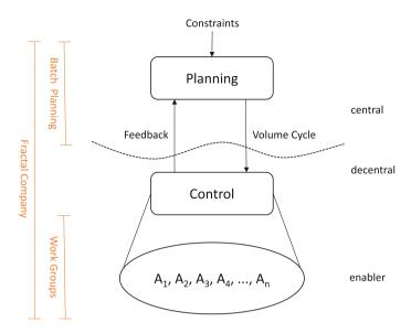
**Fig. 4** Conceptual approach of decentralized planning and control based on CPS. The main basic principles can be found on the *left side* of the figure. The concept of fractal companies represents the thematic framework. Batch planning methods help to define the number of orders handed over to working group consisting of CPS and human workers who organize their tasks
