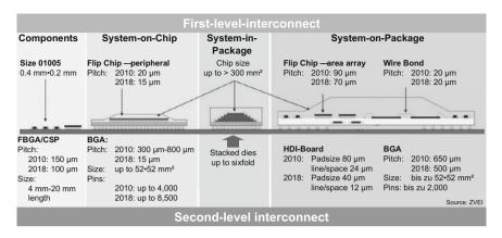
Fig. 2 Miniaturization as a key driver in the development of highly integrated systems in electronic devices [39]
