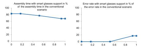
Fig. 8 Reduction of lead time and failure rate by the application of smart glasses as CPAS
