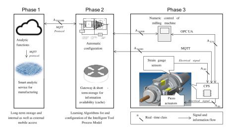
Fig. 6 CPS for milling machines
